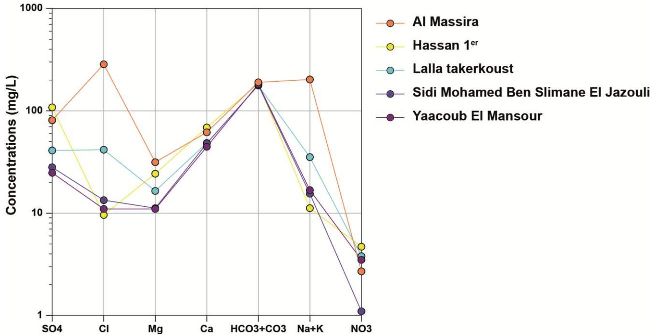
**Figure 3 :** Facies of surface water according to Schoeller-Berkaloff diagram.
