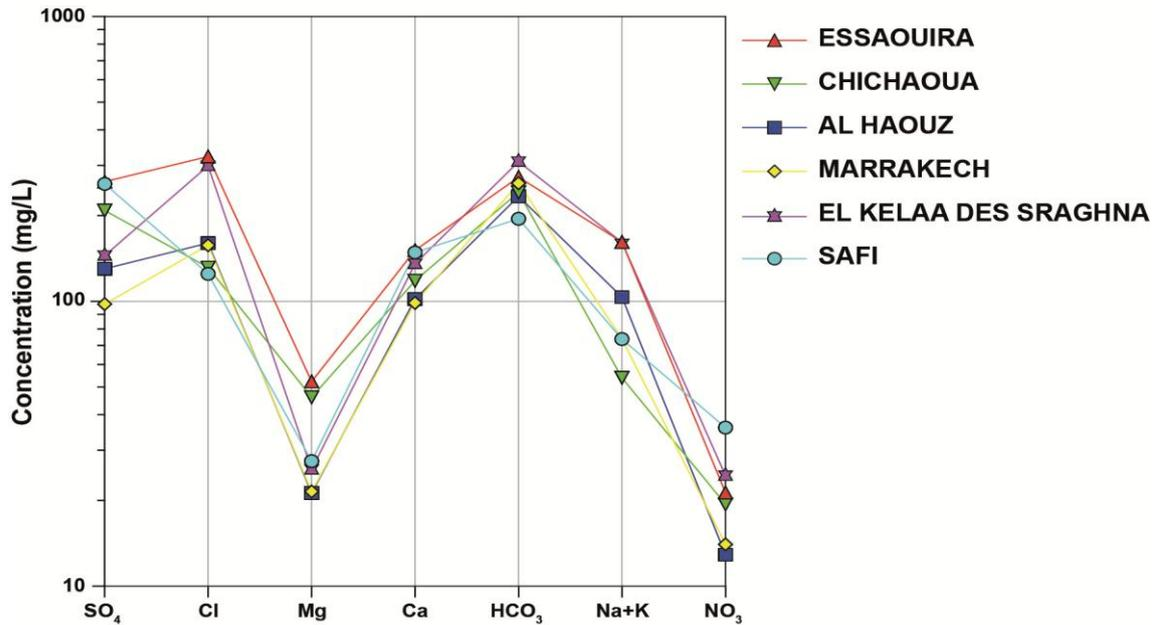
Figure 5 : Facies of groundwater according to the Schöeller-Berkaloff diagram.
