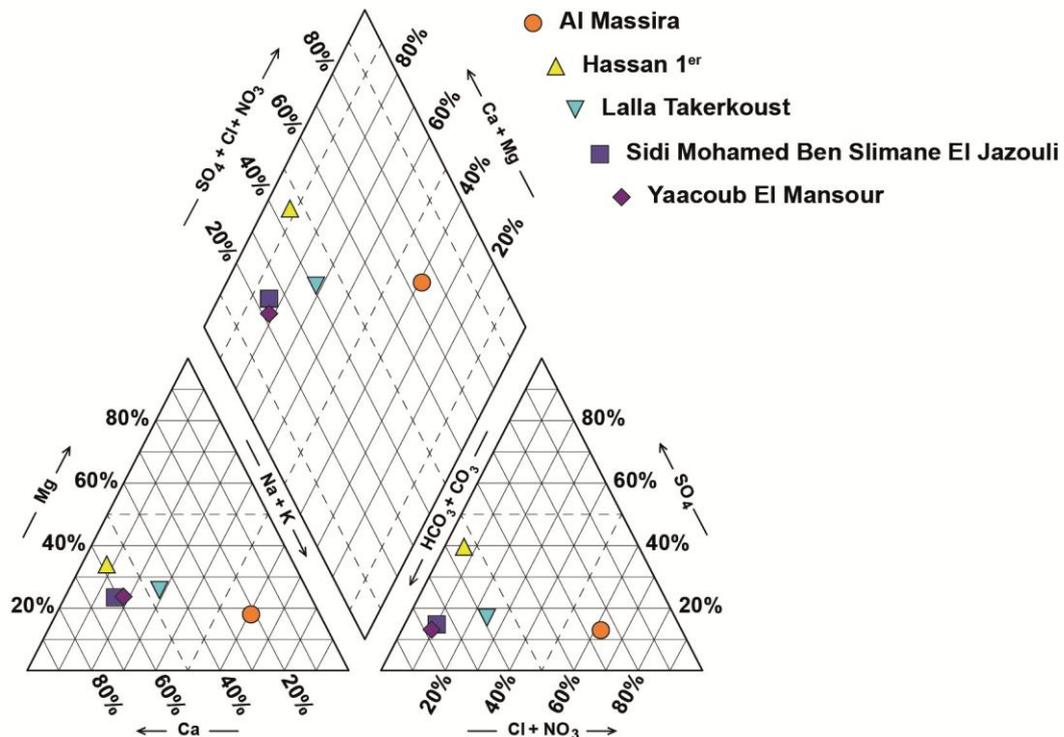
**Figure 2 :** Facies of surface water according to Piper diagram.
